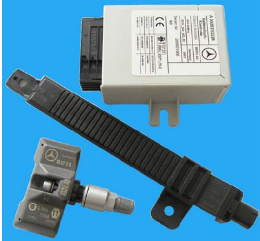
The components of a typical TPMS system: wheel sensor, antenna, and central electronics unit.
