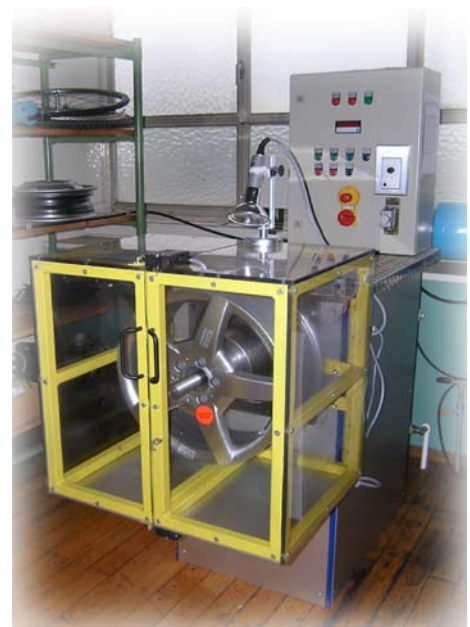
Spin tester to simulate loading on wheel sensor up to 480 km/h
