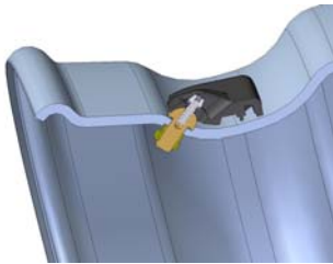
Dowel-type fastening of wheel sensor in the case of insufficient space behind the valve.
