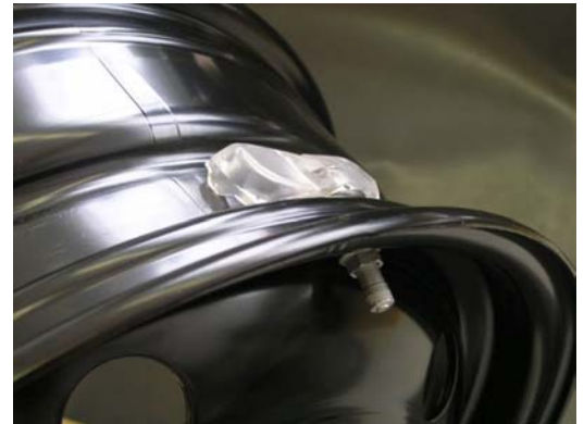
Wheel sensor attached to back end of tire valve
