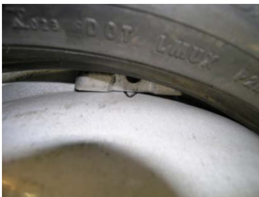
Tire bead sliding over wheel sensor during tire-assembly
